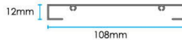
① Front & Back Panel Thickness: 1.3mm
